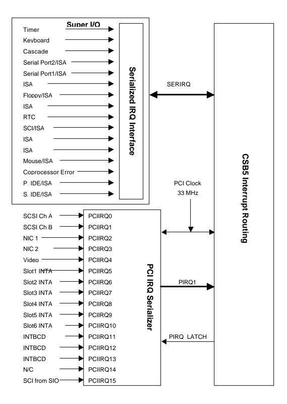
Figure 4. SDS2 Interrupt Routing Diagram
